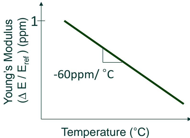
*Elastic Modulus of  $\text{SiO}_2$  vs. Temperature*
