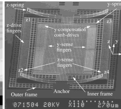
Figure 6: SEM of a released gyroscope.
