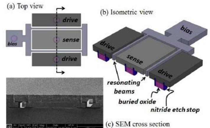
Figure 2: Schematic and cross-sectional SEM images of a DETF resonant thermometer.
