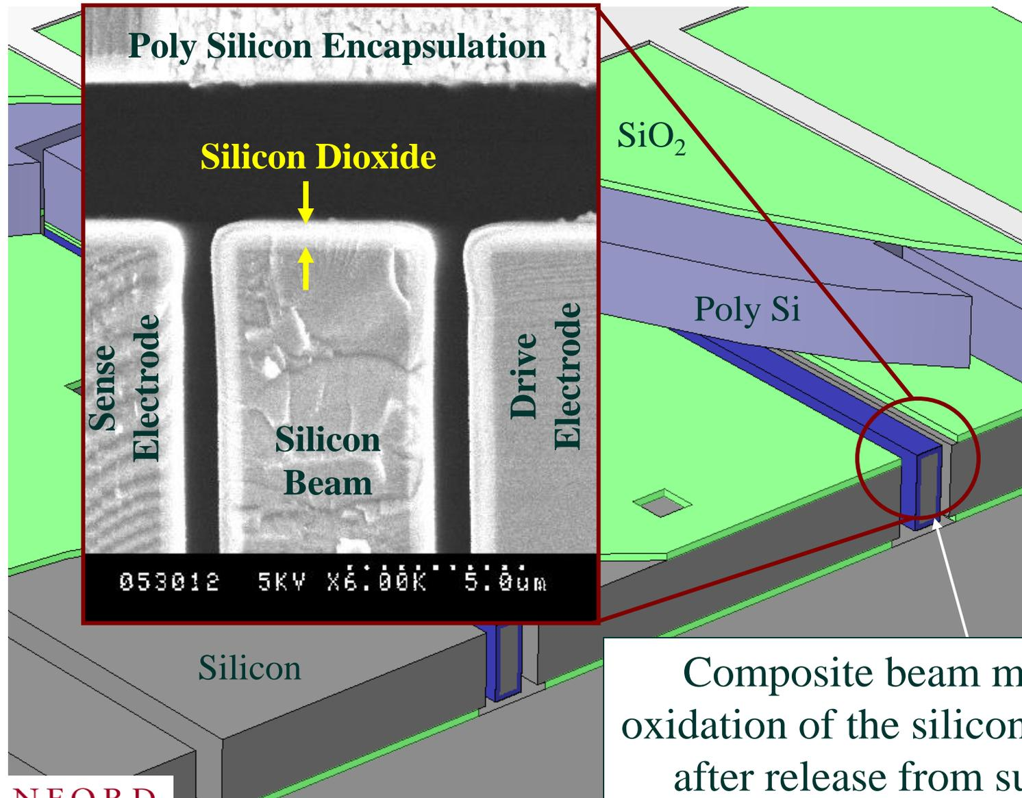
Composite beam made by oxidation of the silicon resonator after release from substrate
