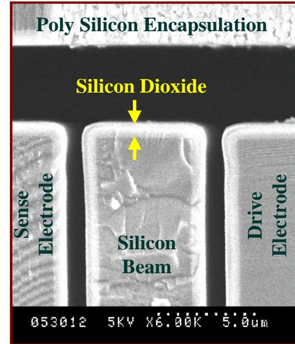
Should provide 20x reduction in frequency error of resonators without any other improvements
