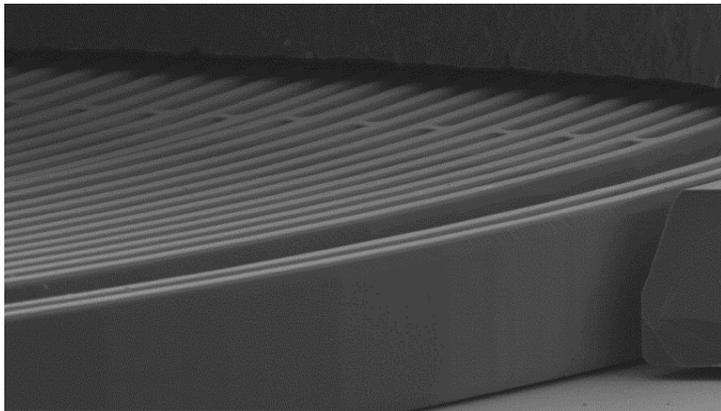
*Since we were making resonant theromometers and accelerometers, we also attempted a prototype wine-glass gyro*
