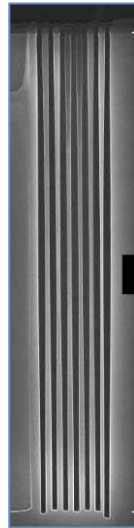
High Aspect Ratio 1.7 x 41 \mu\text{m} 24:1 AR
