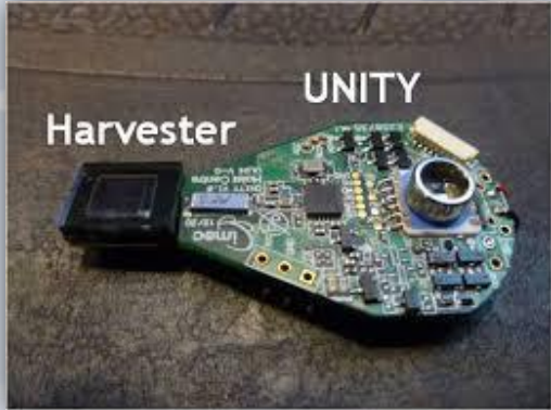
Imec's Autonomous TPMS System ('unity') with Integrated Piezo-electric Energy Harvester
