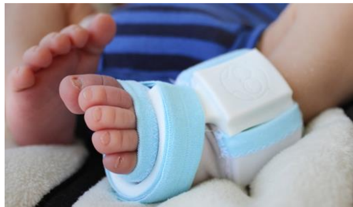
Smart sock from Owlet Baby Care monitors infant's quality of sleep, blood oxygenation levels, and skin temperature
