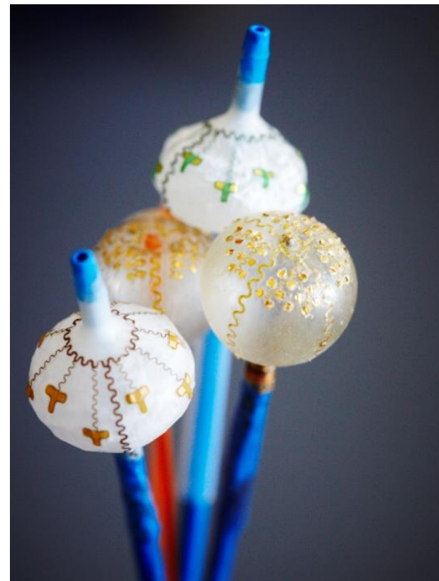
Catheter-tip balloons with flex and stretchable sensors monitoring balloon's performance in the body. MC10
