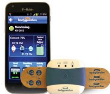
Preventice's smart bandage constantly tracks cardiac ECG and rhythm monitoring
